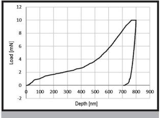
FIG. 2. Nanoindentation load-displacement curve obtained for HAp coating with Ni nanoparticles.
